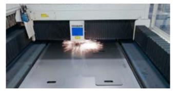
Steel plate laser cutting
