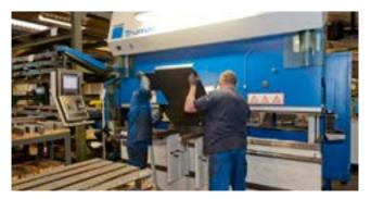
Computer assisted steel plate bending
