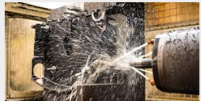
CNC Machining of cast iron saw aggregate
