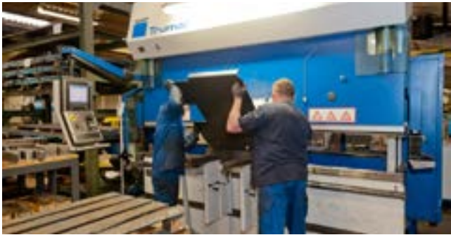
Computer assisted steel plate bending
