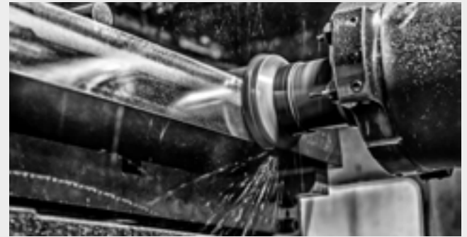
Edge milling of cast iron table
