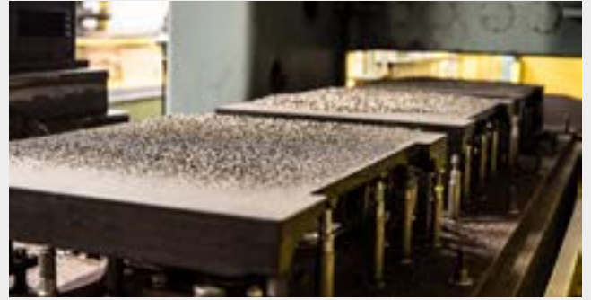
Surface planing of cast iron table
