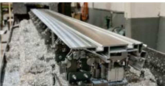
Milling of sliding table surface
