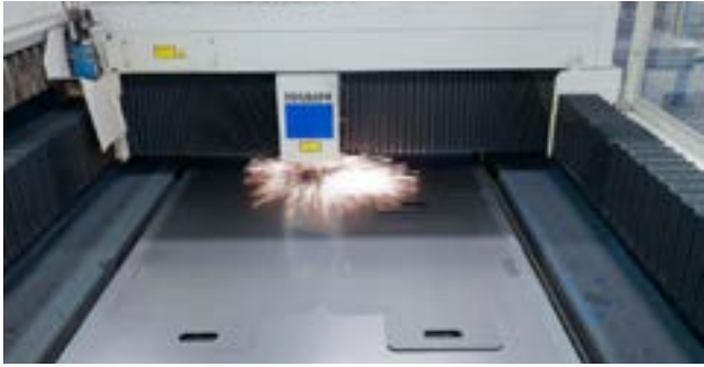
Steel plate laser cutting
